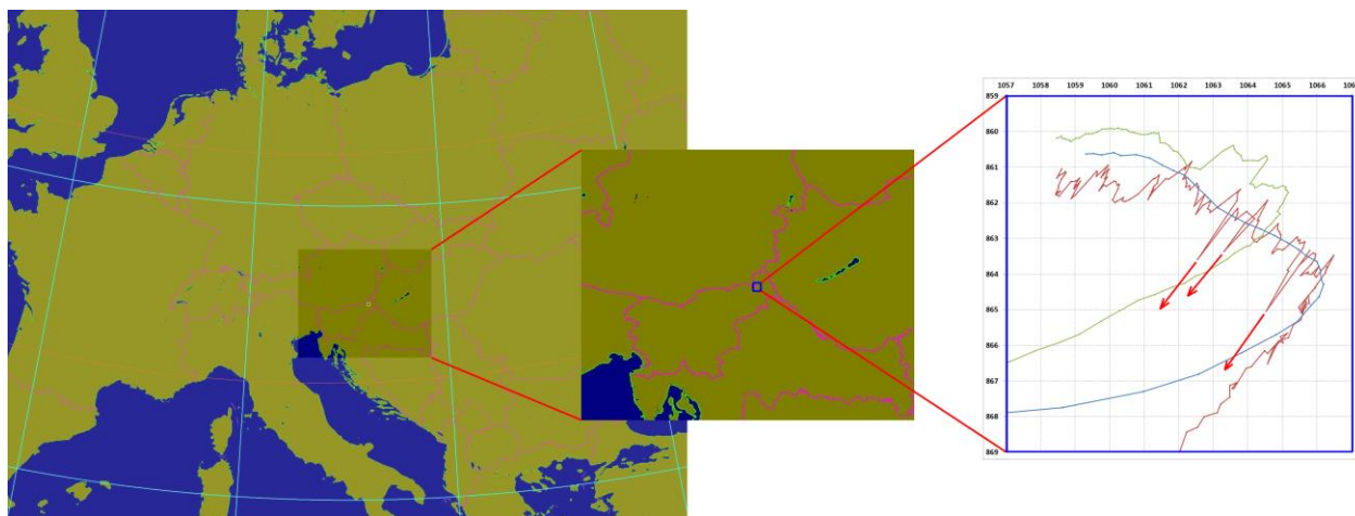
Figure 4: Path of clear air area mass center over image during 17 June 2013 experiment. Red line belongs to MSG-1 2.5-minutes data, green to MSG-2 5-minutes data and blue to MSG-3 15-minutes data.
